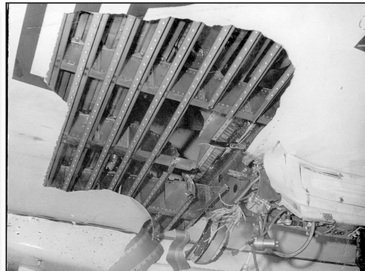
Wing damage to Pete Munro's A-4E 151086, underside.
