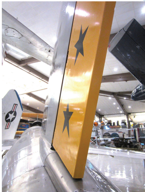
Noticeably thickened rudder of 141828
