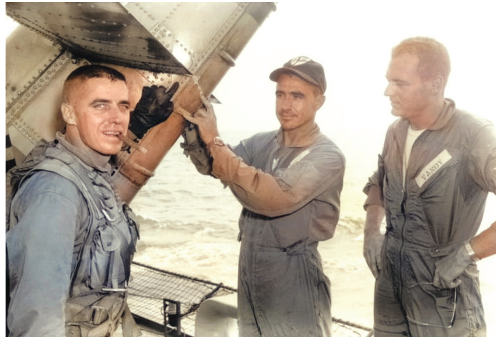
ADJ1 Bowman, LCDR Wetzels and LTJG Vandervelde inspecting bullet hole in tail pylon.
