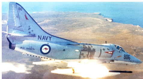
A-4G 886 firing a Zuni rocket. The dark paint areas on the fuselage are corrosion control repairs.
