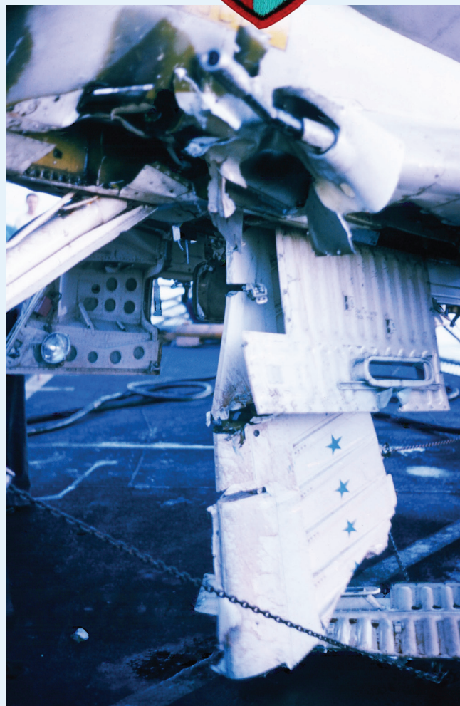
Rudder jammed into main fuel tank after landing.
