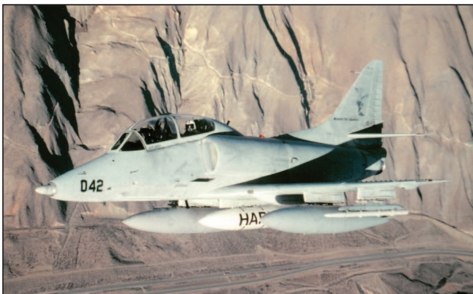
First 2-seater to fly, BuNo 152102 was one of two A-4Es converted to the T-model configuration. Originally designated the TA-4E, designation was quickly changed to TA-4F. Shown here in Jan 1966 as test-bed for HARM missile at China Lake.
