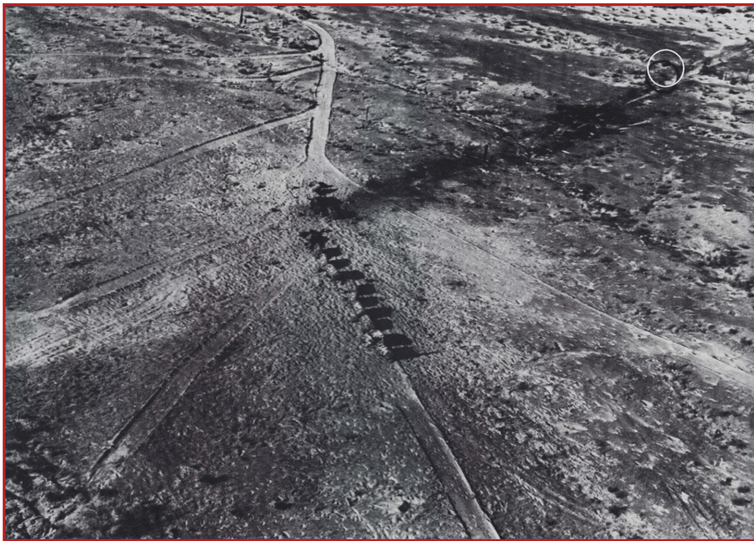
Target-123, a simulated railroad marshalling yard consisting of aircraft engine cannisters to represent railroad tank cars. The Skyhawk cut a long swath along the ground. The circle shows where the pilot landed.
