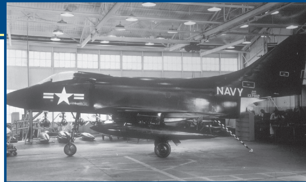
XA4D-1 mockup shows early design configuration of the Skyhawk. (DAC photo.)
