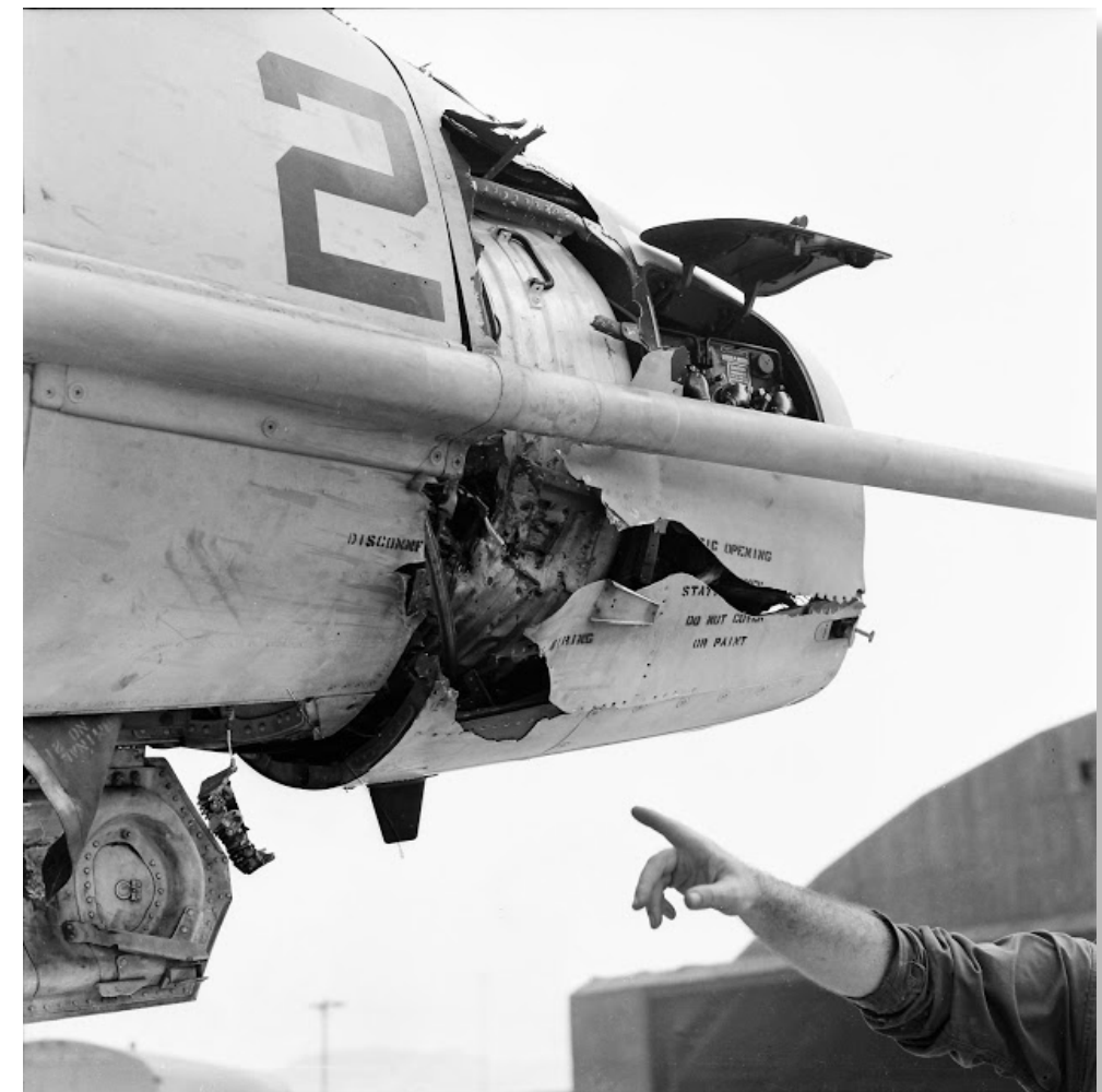
Close-up of nose damage to CDR Gene Tissot’s A-4 Skyhawk at Da Nang. Image from John Rawls via Gary Verver.
