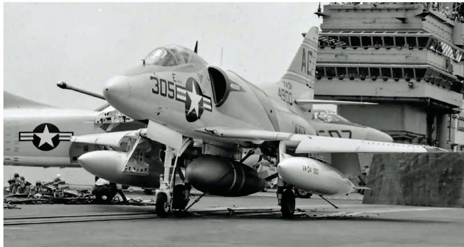
The A-4 was designed from the outset as a nuclear capable aircraft. Here an early Skyhawk sits ready at the catapult carrying a Mark 7 bomb (the U.S.’s first tactical nuclear weapon). EBNAL
