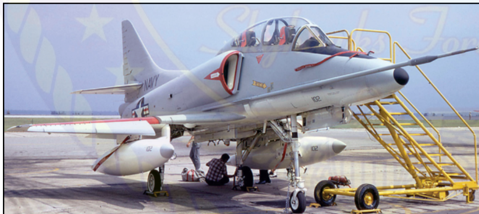
Here is a TA-4E 152102 during a flight test. Note the instrumentation probe on the refueling probe.
