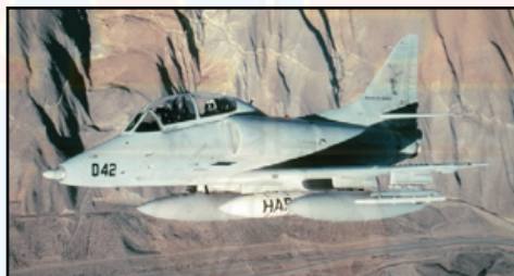
First 2-seater to fly, BuNo 152102 was one of two A-4Es converted to the T-model configuration. Originally designated the TA-4E, designation was quickly changed to TA-4F. Shown here in Jan 1966 as test-bed for HARM missile at China Lake.
