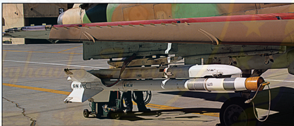
The BVR Systems/IAI MLM EHUD pod is a self-contained AACMI pod while the RADA ACE is an internal system that interfaces with the aircraft's avionics. The IASF leased EHUD pods to equip the Flying Wing Squadron's Ahit jets, as the unit was responsible to the Ahit OTU until 2002. The reassignment of the Ahit OTU mission to the Flying Tiger Squadron coincided with IASF decision to install ACE-II in the Ahit. The illustrated EHUD pod was photographed attached to Ahit N 357 during the Flying Wing Squadron's finale Ahit OTU course in late 2002. (Shlomo Aloni)
