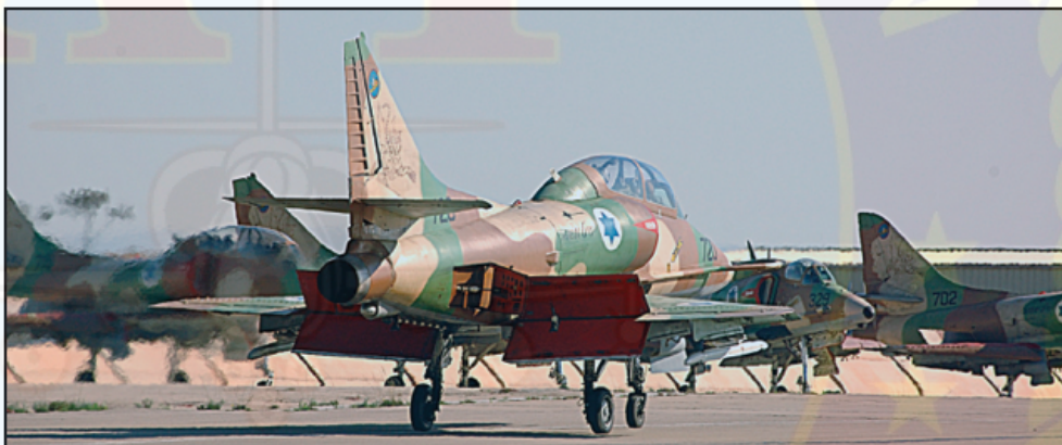
AhitM T 720 taxis to the Last Chance apron at Hatzherim air base to join fellow AhitMs that are already waiting to take-off. The nozzle extension is unique to Israeli Skyhawks and was introduced in 1973 to counter MAN Portable Air Defence System (MANPADS) threats. (Shlomo Aloni)
