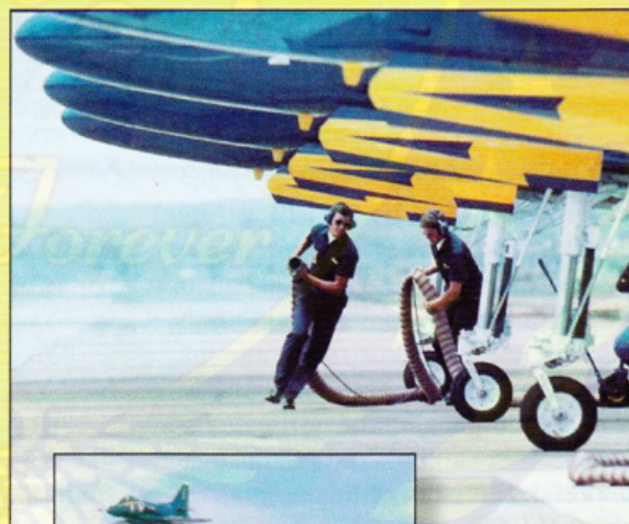
Air starting the A-4s, prior to showtime.
