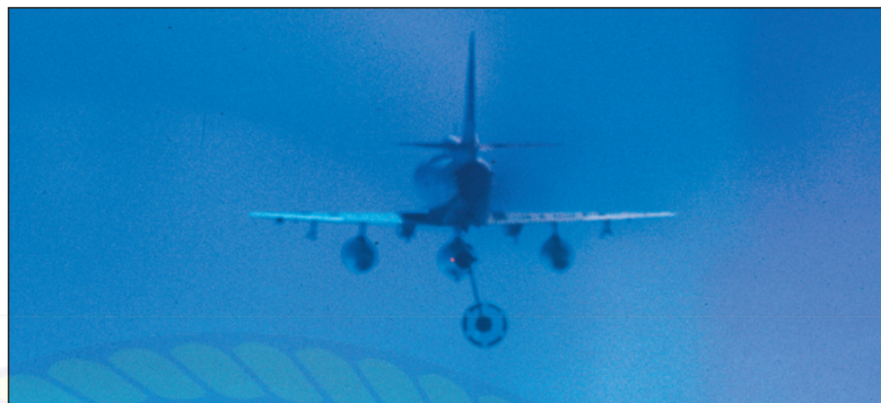
A-4 Buddy Store tanker readies for transfer of fuel to a receiver. The drogue has been extended to the ready position, indicated by the yellow light at left. When a receiver aircraft engages and pushes the hose a few feet into the store, the light changes to green indicating flow of fuel.
