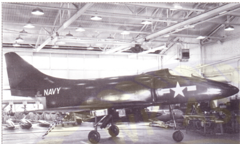
The Initial Mock-Up of the Skyhawk featured an empennage extending beyond the tail pipe. The aft fuselage was later modified to avoid tail buffeting. (Photo from Harry Gann Collection)
