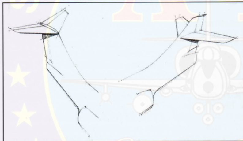
Various Empennage Configurations were envisioned in the initial Skyhawk design phase. (Original sketches from Harry Gann Collection)
